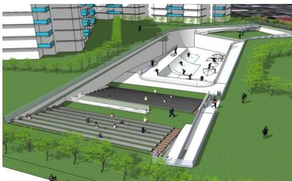
Figure 13. By allocating an area for a sunken open space, it can also serve as a detention pond in cases of extreme rainfall events.
