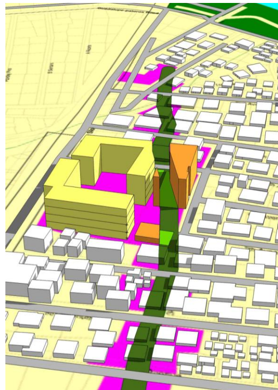
Figure 8. Easement of the West Valley Fault Zone • The drawing shows the buildings including a public school that have been built above the WVF line easement.
